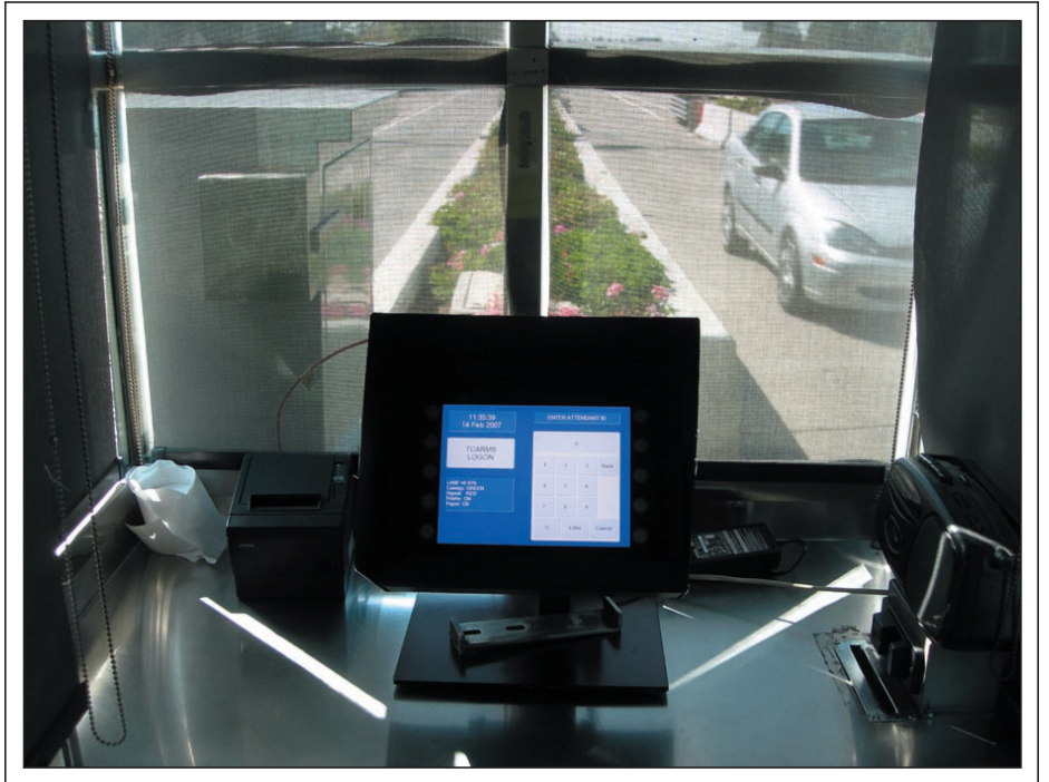
Fig. 8: A tollbooth terminal with an InfiniTouch™ touch panel, where it is subject to repeated touches by the tollkeeper. Resistive touch panels in the previous monitor frequently failed due to extreme wear. The clarity of the touch panel contributes to the contrast of the display in the sunlit booth.
