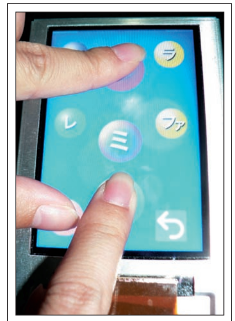
Fig. 5: Sharp's 3.5-in. LCD with in-cell light-sensing optical touch. Photo courtesy of Nikkei Business Publications Tech-On!
