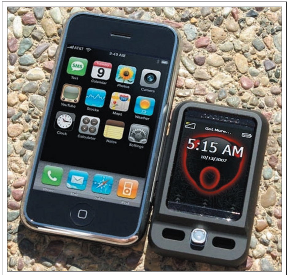
Fig. 2: The Apple iPhone with projected-capacitive touch (left) and the Neonode N2 cell phone with conventional optical touch (right). Photo courtesy of PenComputing.com.
