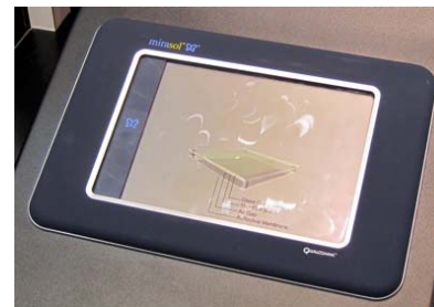
RPO waveguide infrared in prototype 13.3" notebook from LG Displays (2010)
