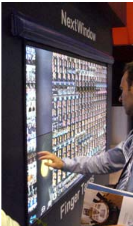
Orion's tiled 84-inch plasma display using NextWindow's optical touchscreen and an amazing demo application from Content Interface (not Fingertaps)
