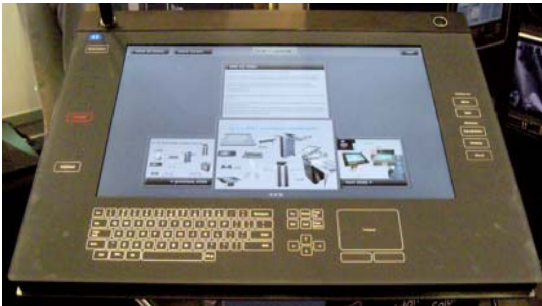
Lectern using Sensitive Object's acoustic touchscreen for zero-bezel effect with many soft-keys around the LCD
