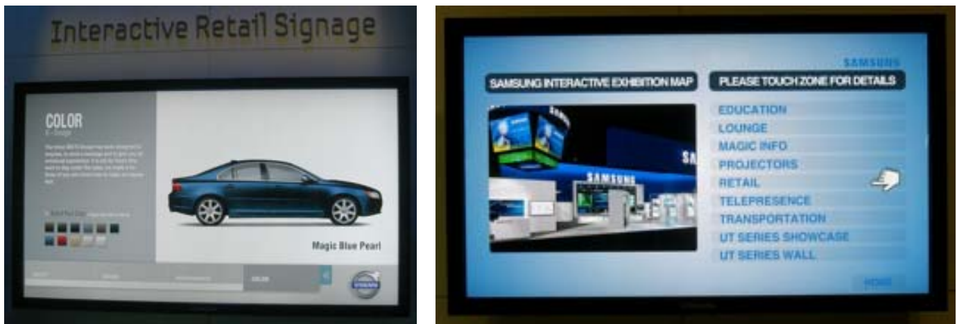
Samsung's 85-inch interactive digital retail sign (left); Samsung's 65-inch interactive wayfinder sign (right), both with traditional IR touchscreens
