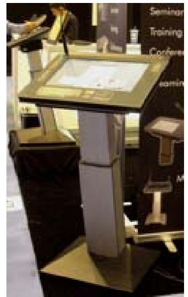
Lectern using Sensitive Object's acoustic touchscreen for zero-bezel effect with many soft-keys around the LCD
