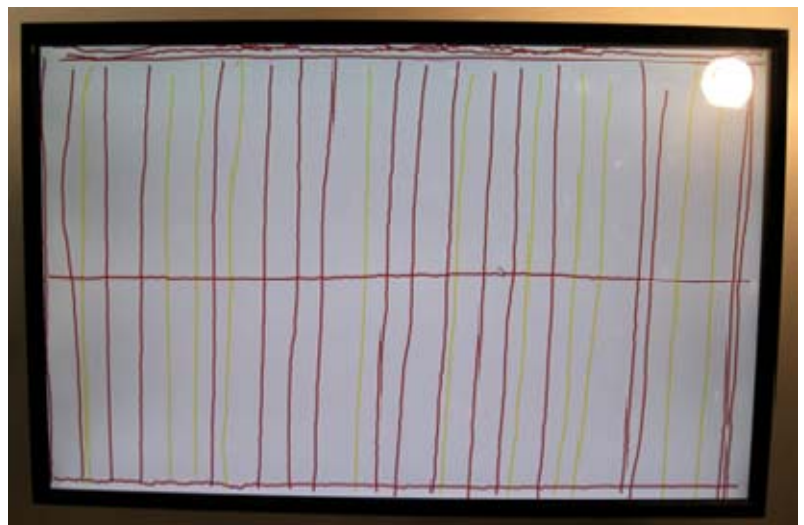
3M’s 19.0-inch projected-capacitive 10-touch monitor (note noise in lines drawn along upper edge)
