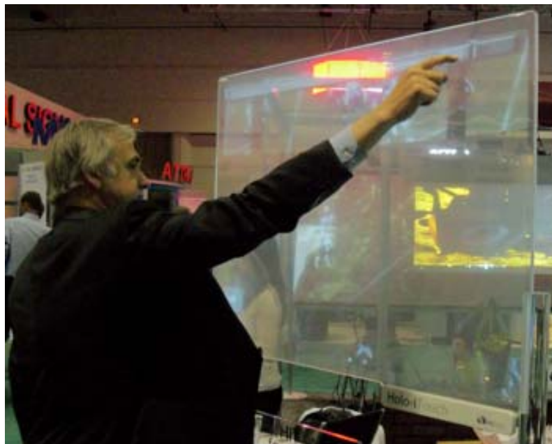
Vislogix's "Holo-iTouch" using Visual Planet's projected-capacitive film
