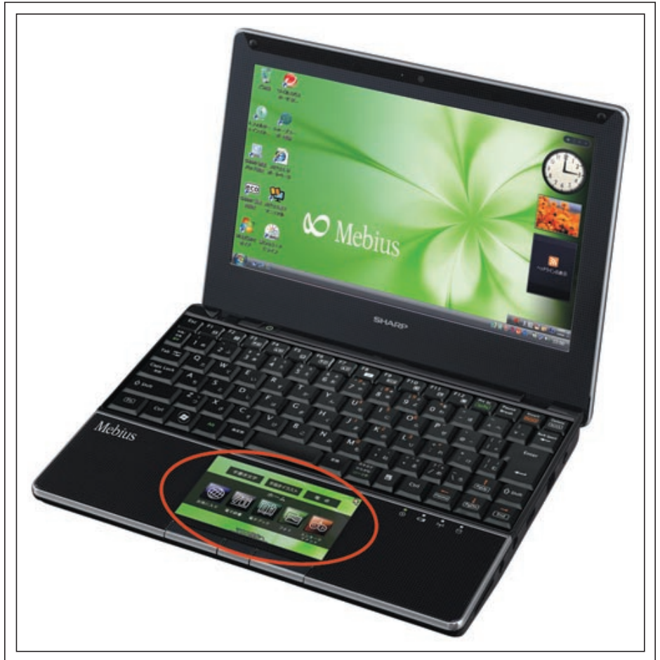
Fig. 2: Sharp’s PC-NJ70A netbook is the first commercial product to use any form of in-cell touch. A light-sensing, in-cell touch screen is integrated in the touchpad LCD, circled in red in the photograph. Source: Sharp.
