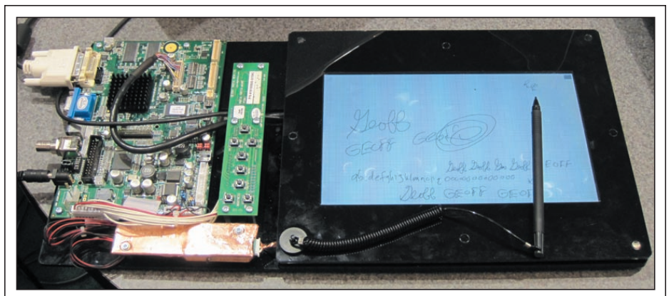
Fig. 2: Above is Stantum’s very-high-resolution (0.65 mm) analog multi-touch resistive (AMR) touch screen, showing extremely fine digital ink. The touch screen uses four Sitronix controller chips around the edge (under the bezel). The left side of the photo is a standard video card used to drive the electronics on the right.
