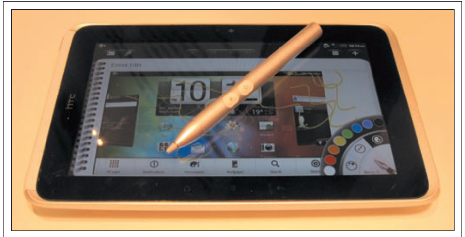
Fig. 3: The HTC Flyer Android tablet with a 7-in. display and N-trig's dual-mode (pen and finger) pro-cap touch screen. With the product thickness at only 0.5 in., there is no internal storage for the stylus. Photo courtesy Geoff Walker.
