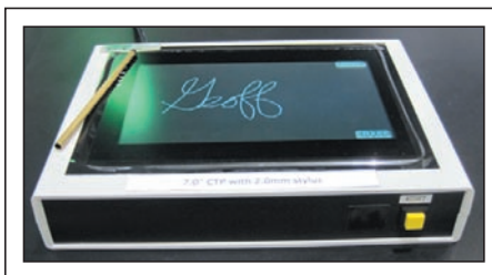
Fig. 7: A 7-in. p-cap touch screen from Emerging Display Technologies supports a passive stylus with a 2-mm tip. The author wrote his name on the screen with palm contact; there were no spurious points recorded and the ink was noise-free with normal stair-stepping that software could easily smooth. Source: Geoff Walker.
