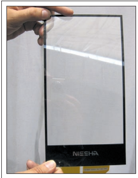
Fig. 6: Stantum's latest digital-resistive (iVSM) touch screen uses Peratech's "quantum tunneling" pressure-sensing material in a layer only a few microns thick between the film and the glass. Note the Nissha branding; Stantum and Nissha Printing have partnered to produce a line of "Fine Touch Z" touch screens in sizes 5–12 in. Source: Geoff Walker.
