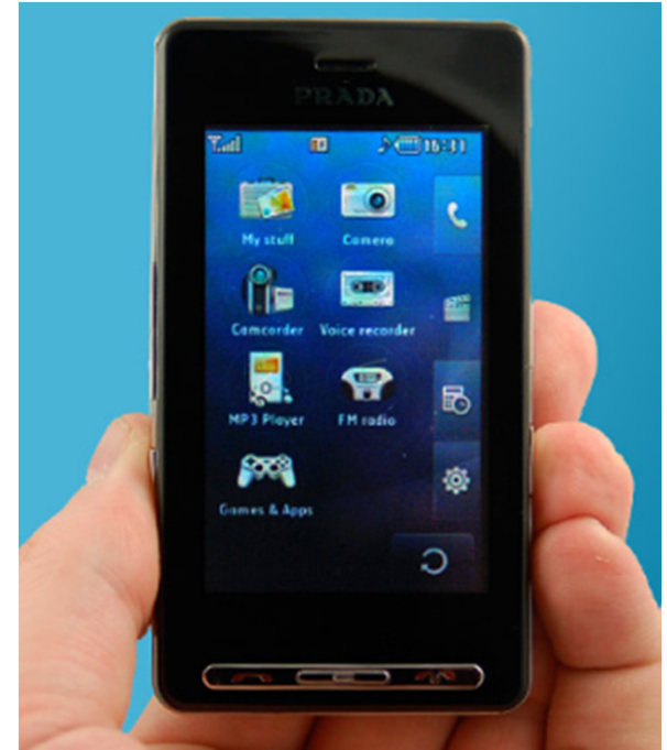
LG-Prada mobile phone with Synaptics' projected-capacitive touch-screen; launched 3 months before iPhone
